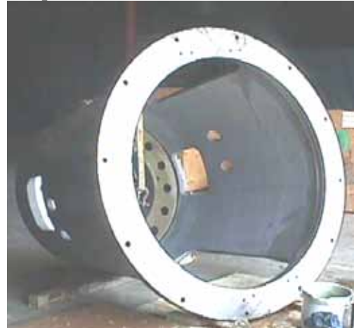
Recirc Pump Case - Box 2 of 6
